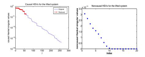
Figure 6: (a) Causal Hankel singular values for original and reduced-order lifted systems. (b) Noncausal Hankel singular values for original and reduced-order lifted systems.
