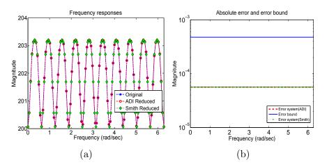
Figure 4: (a) The frequency responses of the original and the reduced-order lifted systems; (b) absolute error and error bound.
