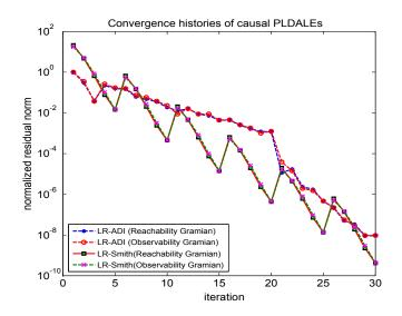
Figure 2: Normalized residual norms for the causal reachability and observability lifted projected Lyapunov equations.
