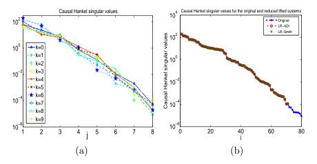
Figure 3: (a) Causal Hankel singular values for subsystems; (b) Causal Hankel singular values for original and reduced-order lifted systems.
