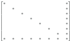
Figure: arrowhead matrix pattern and connectivity graph.
