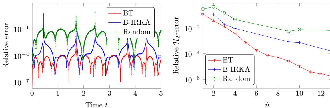
Figure 2: Relative error of heat transfer model ( $n = 225$ ) to an input  $u(t) = (\cos(\pi t), \cos(2\pi t))^T$  and relative  $\mathcal{H}_2$ -error for balanced truncation, B-IRKA and randomly chosen initial points.
