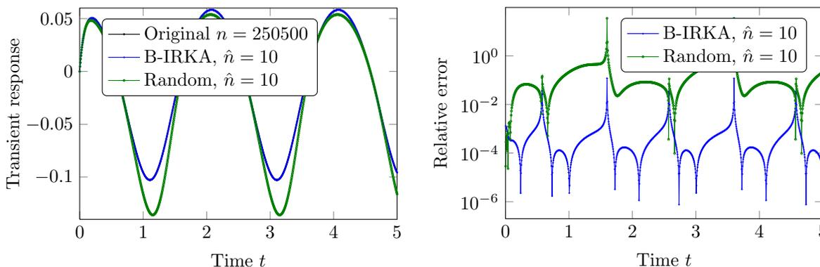
Figure 3: Transient response and relative error of heat transfer model ( $n = 250500$ ) to an input  $u(t) = (\cos(\pi t), \cos(2\pi t))^T$  for B-IRKA and randomly chosen initial points.
