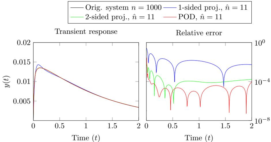
Figure 1: **A nonlinear RC circuit.** Comparison of moment matching methods and POD subject to boundary control  $u(t) = e^{-t}$ .
